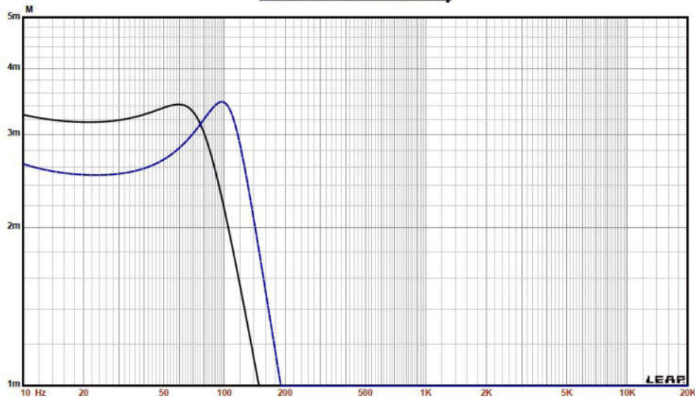
Figure 4: Cone excursion curves for the 9 V/14 V curves shown in Figure 2.
