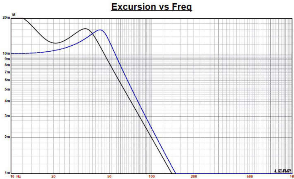
Figure 4: Cone excursion curves for the 33 V and 34 V curves shown in Figure 2.
