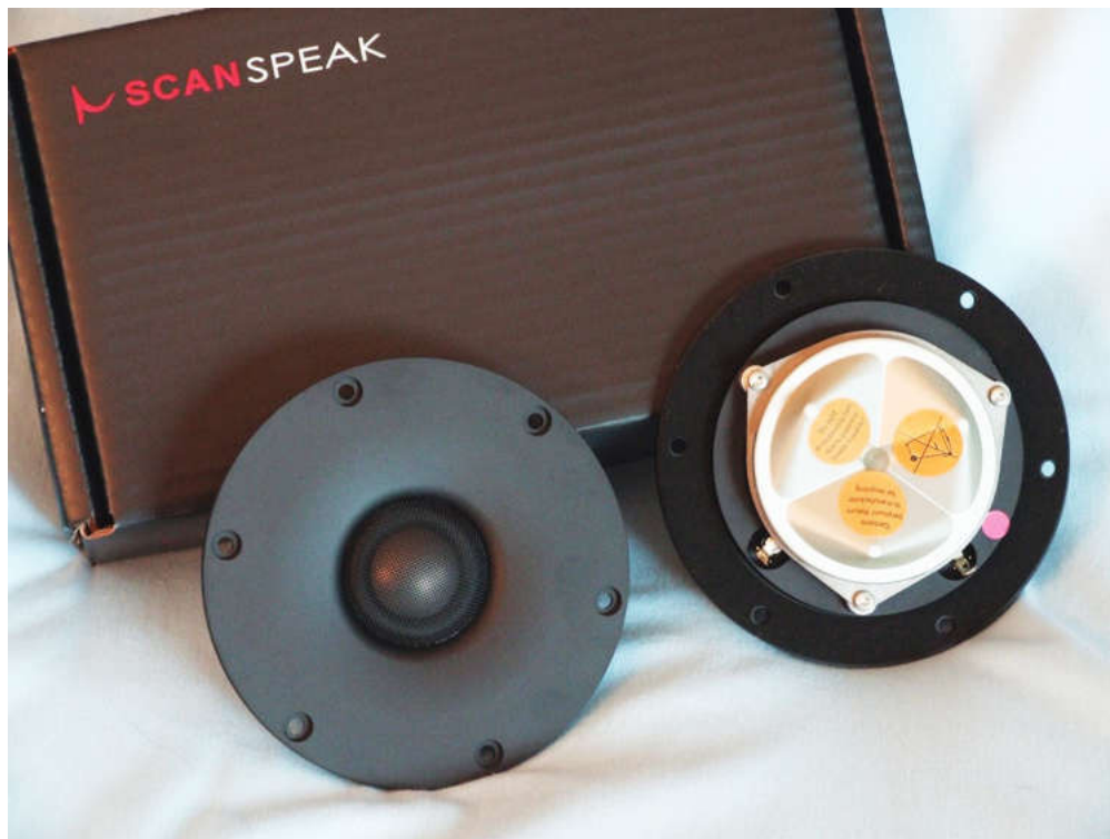
Photo 1: Scan-Speak released the D2908/714000, a 30-mm beryllium dome tweeter.
