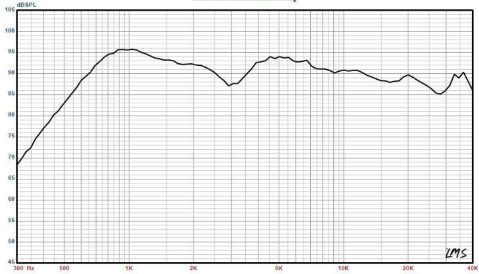
Figure 2: Scan-Speak D3004/604000 on-axis response.
