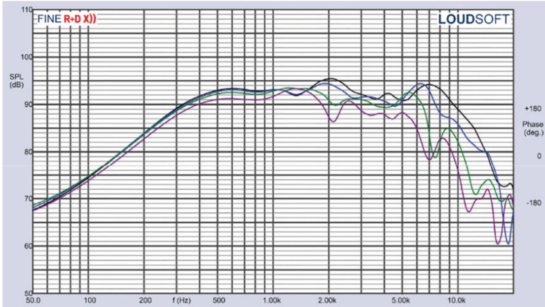
Figure 3: Scan-Speak Ellipticor D8404/552000 horizontal on- and off-axis frequency response (0°=black; 15°=blue; 30°=green; 45°=purple)
