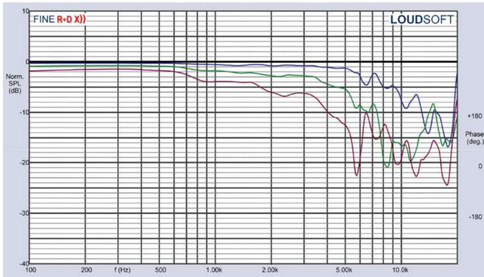
Figure 12: Purifi PTT5.25X-NFA-01 normalized on- and off-axis frequency response (0°=black; 15°=blue; 30°=green; 45°=purple).
