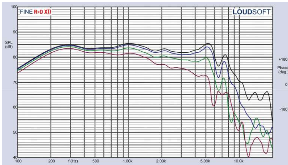
Figure 11: Purifi PTT5.25X-NFA-01 horizontal on- and off-axis frequency response (0°=black; 15°=blue; 30°=green; 45°=purple).
