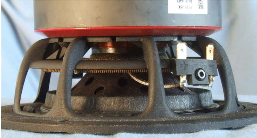
Photo 2: Close-up view of the Purifi PTT5.25X-NFA-01 motor/cone assembly.
