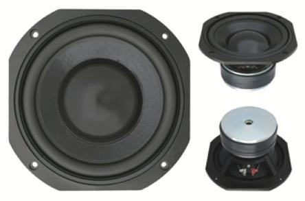
The SB220.1 has been optimised for bass performance in sub-woofer applications. It uses a vented, symmetrical field magnet system with an exceptionally long voice coil for large linear excursion capability. The cone uses a long fibred pulp for rigidity and with the dustcap, is damped by a coat of glossy black dope. Suspension stiffness and excursion is optimised for tight control over high power transients.
