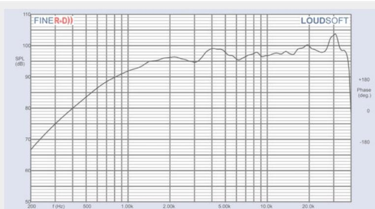
Figure 2: BlieSma T34B-4 on-axis frequency response.
