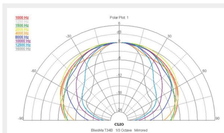
Figure 5: BliesMa T34B-4 180° horizontal plane CLIO polar plot (in 10° increments).
