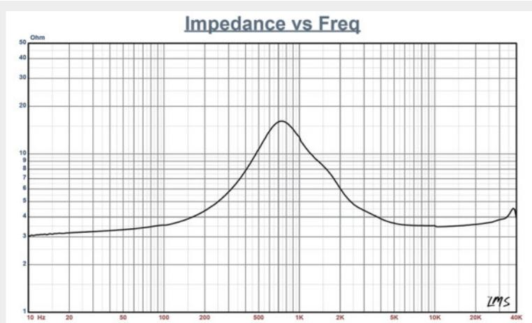
Figure 1: BlieSma T34B-4 impedance plot.
