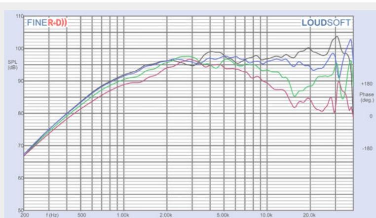
Figure 3: BlieSma T34B-4 horizontal on- and off-axis frequency response (0° = black; 15° = blue; 30° = green; 45° = purple)
