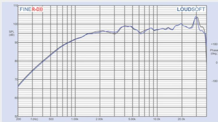
Figure 6: BlieSMA T34B-4 two-sample SPL comparison.
