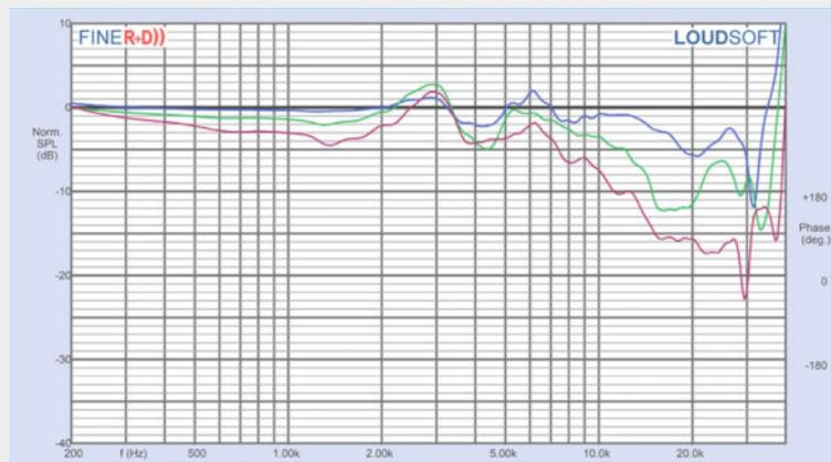
Figure 4: BliesMa T34B-4 normalized on- and off-axis frequency response (0° = black; 15° = blue; 30° = green; 45° = purple)
