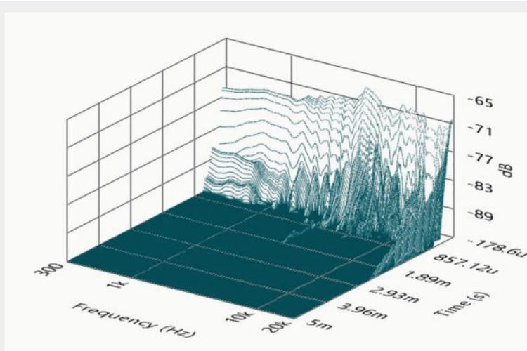
Figure 7: BlieSMA T34B-4 SoundCheck CSD waterfall plot.
